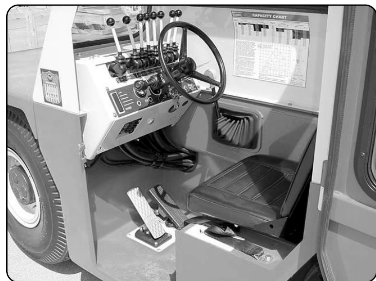
Ergonomic controls directly connected to valve with simultaneous function operation
