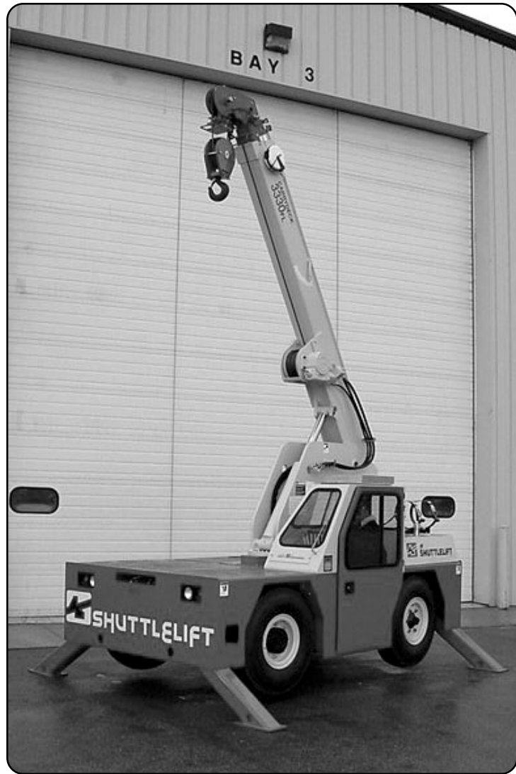
Single stage outriggers for operation in confined areas. 3330FL shown with optional cab.
