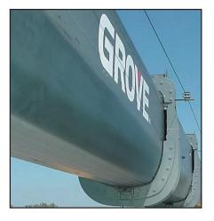
36 - 110 ft. (11 - 33.5 m) four section full power sequenced synchronized MEGAFORM<sup>™</sup> boom designed for maximum vertical and lateral strength
