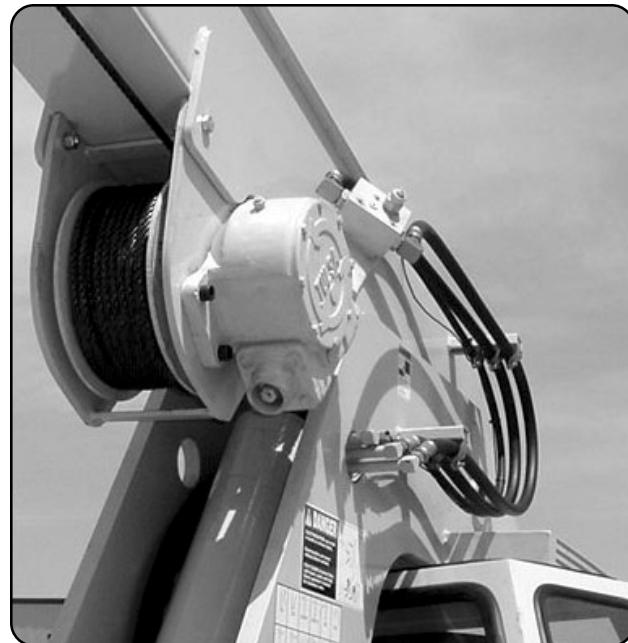
Large winch capacity for use with 1/2" (12.7 mm) wire rope
