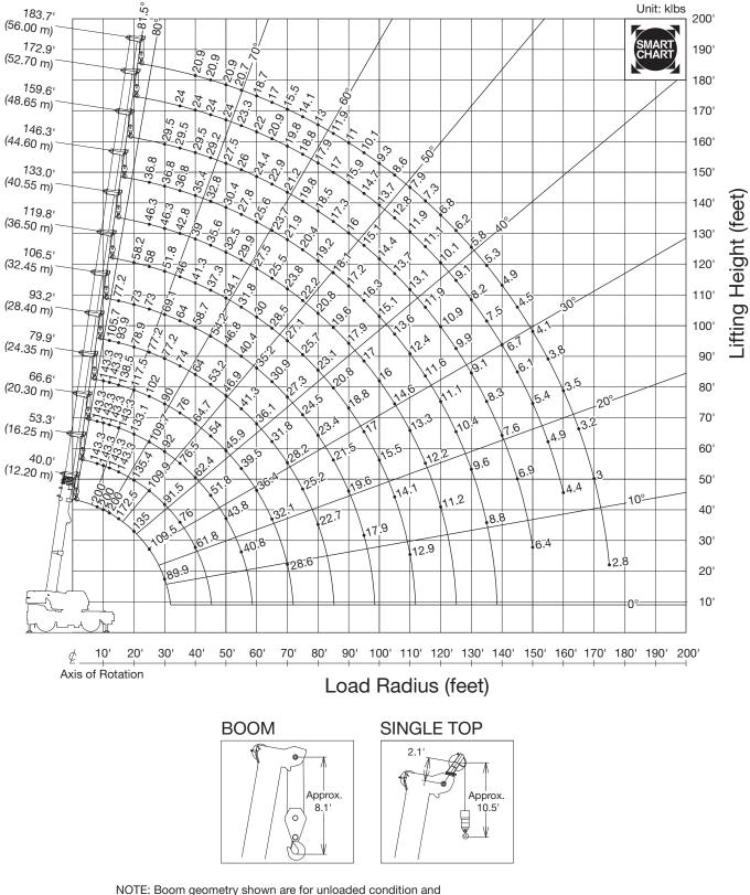
MOTE: Boom geometry shown are for unloaded condition and machine standing level on firm supporting surface. Boom deflection and subsequent radius and boom angle change must be accounted for when applying load to hook.
