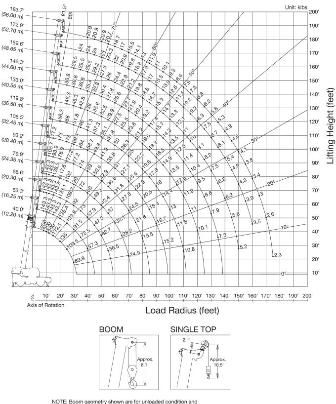
machine standing level on firm supporting surface. Boom deflection and subsequent radius and boom angle change must be accounted for when applying load to hook.
